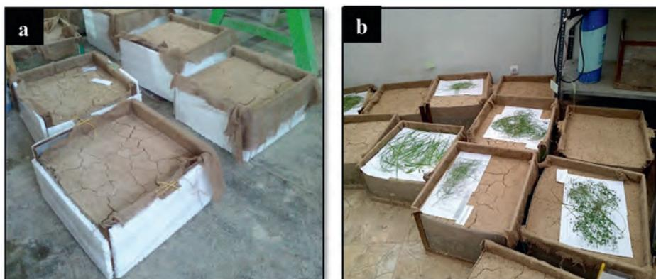
Fig. 6. Cracked soil surface of the control and treated plots after undergoing a FT cycle.
