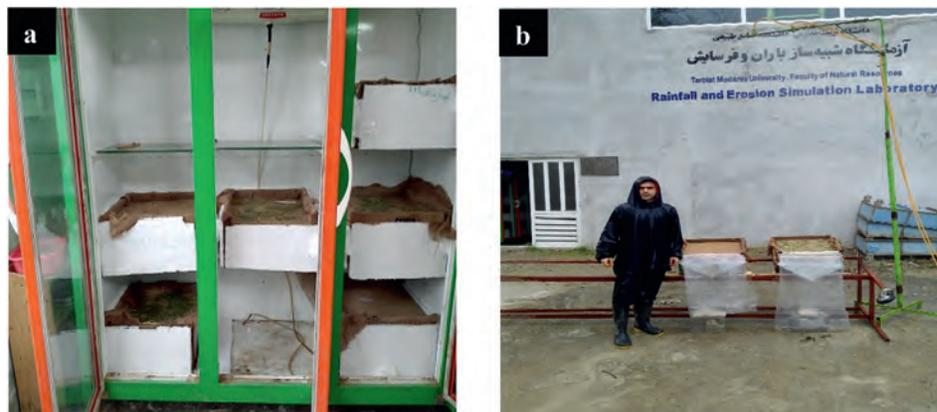
**Fig. 2.** Simulation of the study FT cycle in designed cooling system (left), and rainfall simulation and runoff measurement (right).
