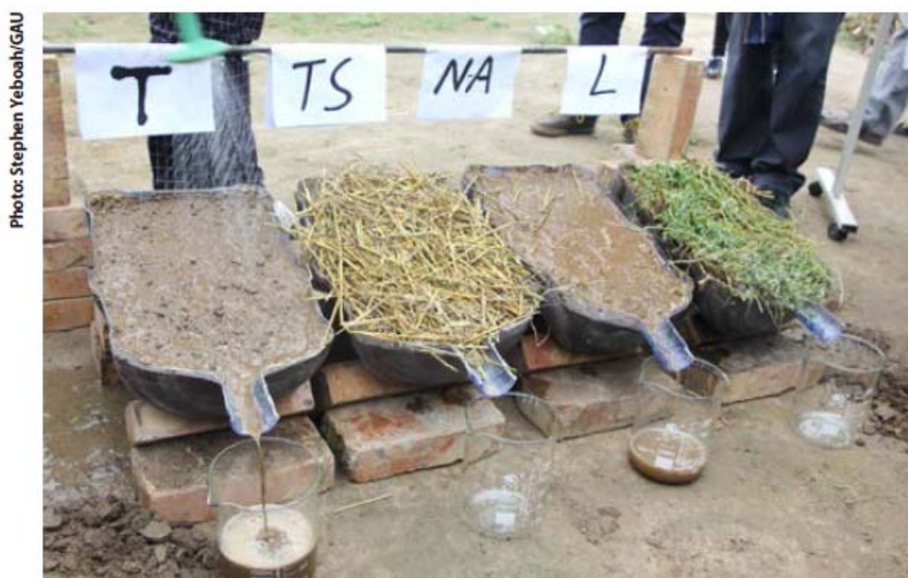
▲ Runoff in action during the rainfall simulation on tilled soil (T), tilled soil with straw cover (TS), non-agricultural soil (NA) and recently mowed lucern (L).
