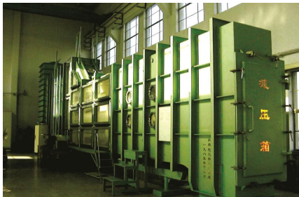
Vacuum Tank (Vacuum Percentage 98.7%, Flow Discharge 1.0 m 3 /s)
