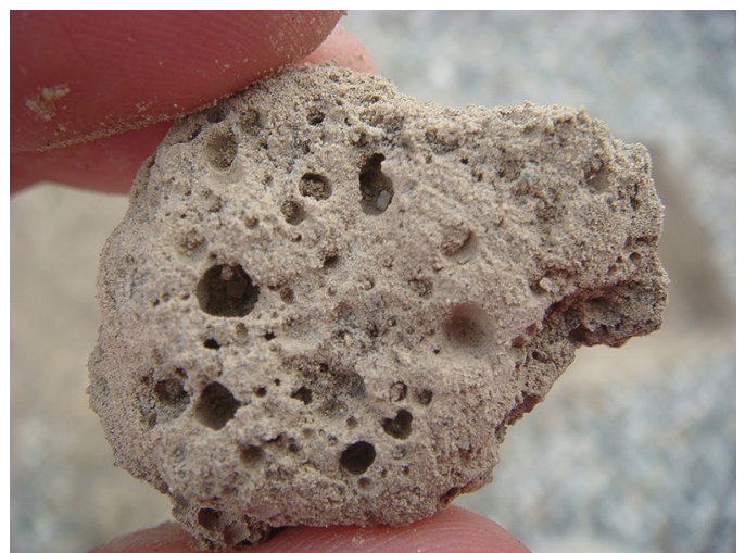
This chunk of soil has numerous vesicular pores, which are spherical and look a bit like bubbles. Credit: Judith Turk
