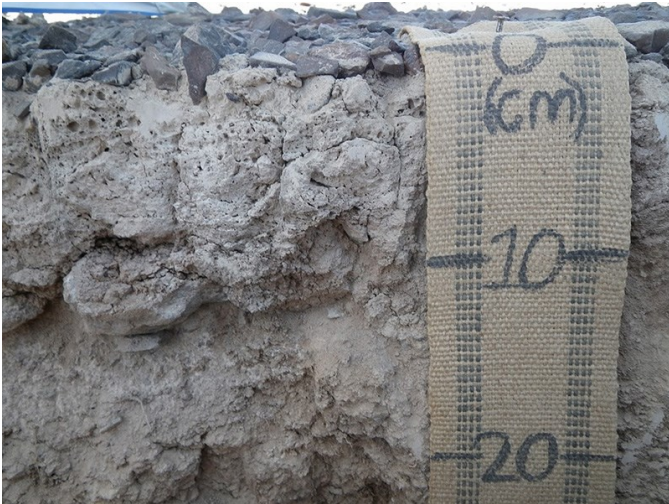
This soil profile shows the vesicular horizon in a research plot near Mina, NV. Credit: Judith Turk.
