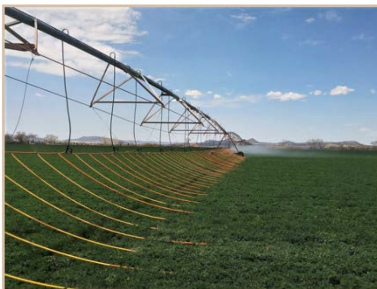
Advanced pivot irrigation systems such as mobile drip irrigation, low-energy precision application and low-energy spray application reduce wind drift and evaporation - allowing for reduced irrigation rates. Photo credit: Jonathan Holt
